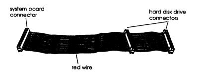
The ribbon cable has a red wire running down one side, a system board connector at one end, and two drive connectors near the other end.
